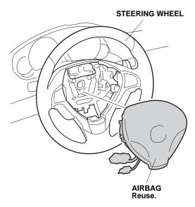
11. Unplug the 20-pin connector from the cable reel. Remove the steering wheel bolt. Using a steering wheel puller, remove the steering wheel. Do not thread the steering wheel puller bolts in more than 10 mm. Be careful not to rotate the steering wheel during removal.
