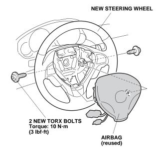
31. Install two new TORX bolts. Torque the TORX bolts to 10 N·m (3 lbf-ft).
