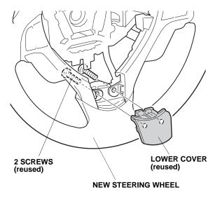
25. Install the steering wheel cover to the new steering wheel using four screws.
